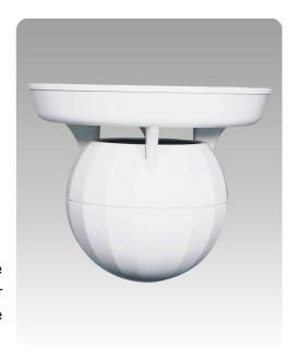
The built-in 6" full range speaker driver is designed of wide frequency response 100-13kHz, the multiple power taps of 7.5W, 10W, 15W, 20W, 30W & 60W could meet different applications varies from room size and ambient noise surroundings.
