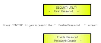
Once a Password has been entered into the WS-P26 through the steps described in the previous paragraph, it is possible to "Enable" or "Disable" the password function and therefore lock the WS-P26 restricting access to all functions.
